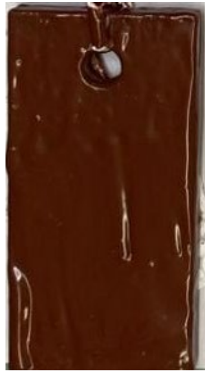
Epoxy coated coupon
