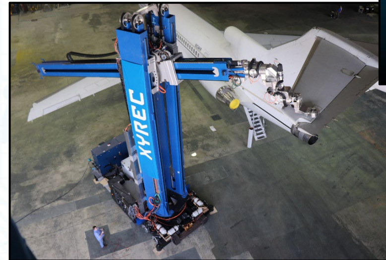
Laser ablation (depaint) robot used for large-scale industrial contexts
