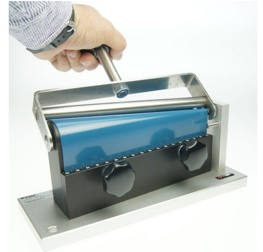
ASTM D522 Conical Bender in action with panel
