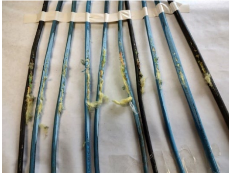
Irrad X-Link (Fail @ 50 Cycles)
