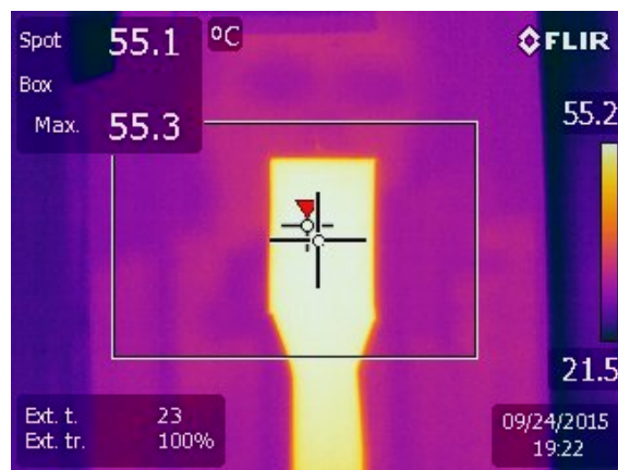
Figure 8 Blackbody Mask Simulating Cable Lug
