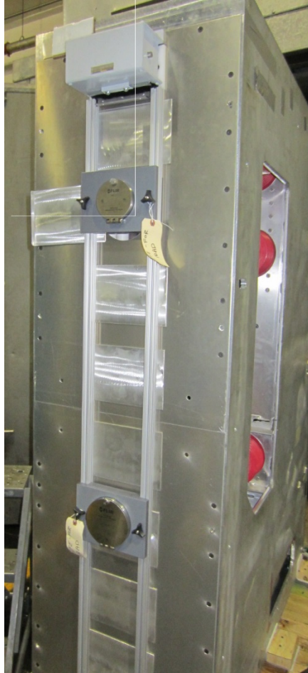
Figure 30 3 and 4 Inch Windows Installed
