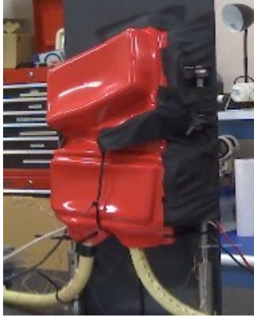
Figure 20 Boot Material Jury Rigged over Heated Lug
