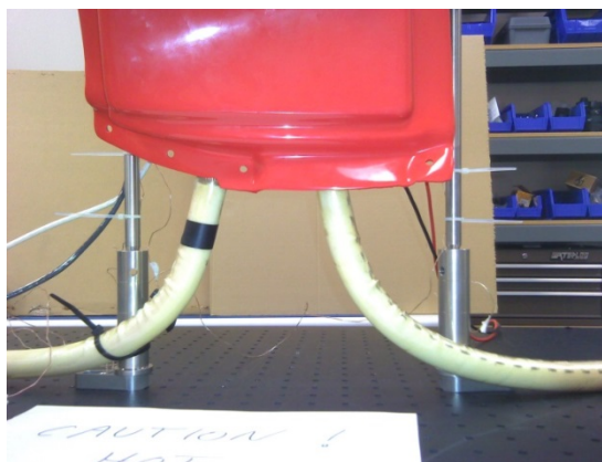
Figure 23 Dust Boot Material Over Heated Lugs
