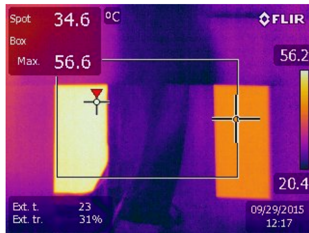
Figure 13 Thermal Image, Two Targets 20°C Apart, FLIR Window
