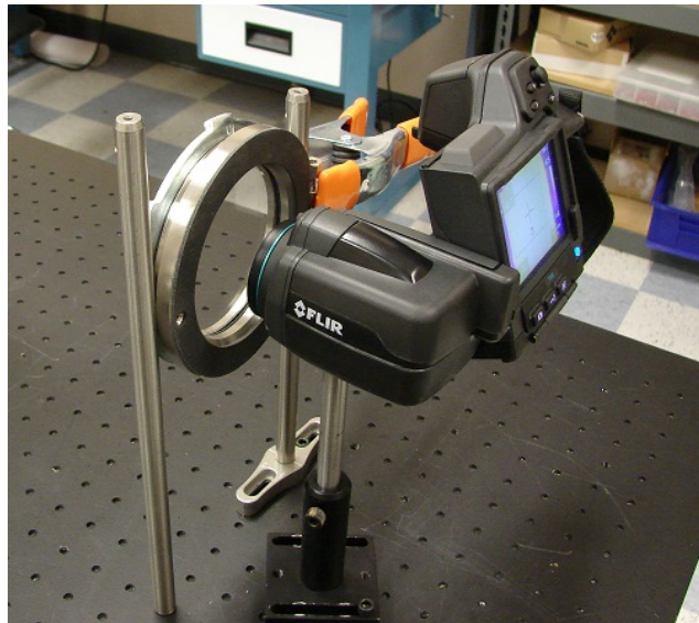
Figure 1 Camera and Window Holding Fixtures
