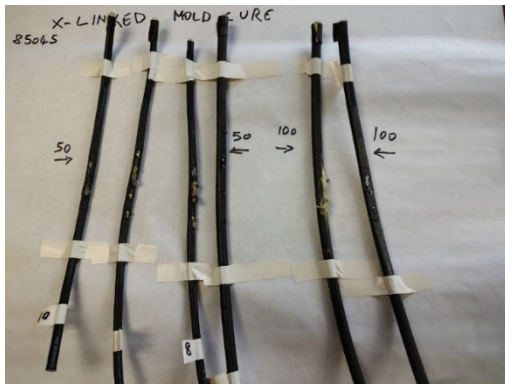
Mold Cure X-Link (Fail @ 50 to 100 Cycles)
