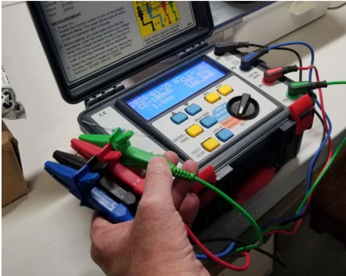
4 Wire, Low resistance meter to measure contact resistance
