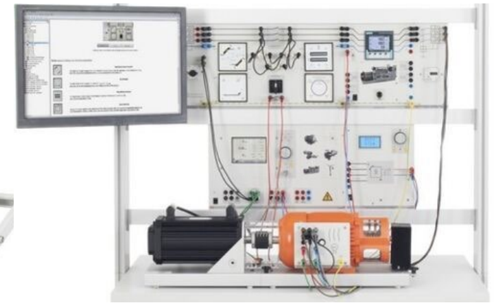
Lucas-Nuelle: EUG1 Manually Operated Synchronous Circuits
