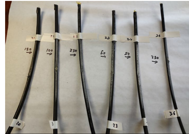
Thermoplastic (Fail @ 50 to 250 Cycles)
