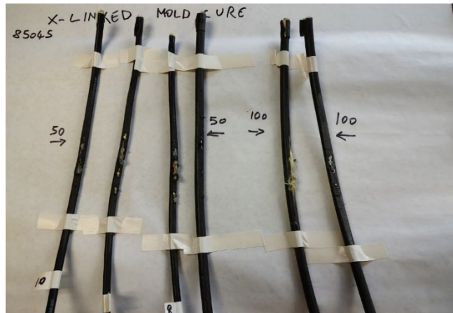
Thermoset Mold Cure X-Link (Fail @ 50 to 100 Cycles)
