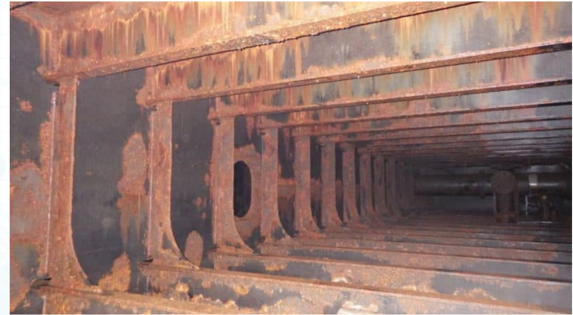
Example corroded ballast tank
