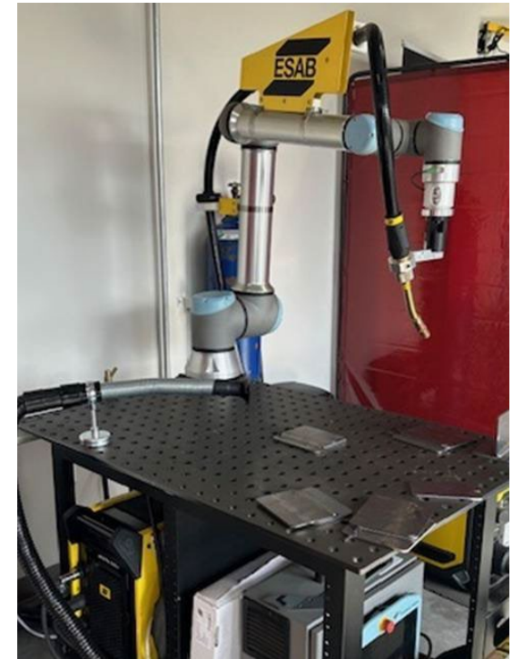
ESAB Smoot CoBot 500I x Power source, U8 Robust Feeder, URIO TT Arm
