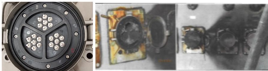
Figure 1 Healthy connector (left). Connector after arc flash event (right)
