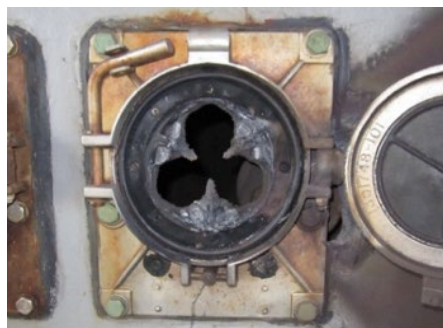
Figure 15 Damage from connector arc flash event
