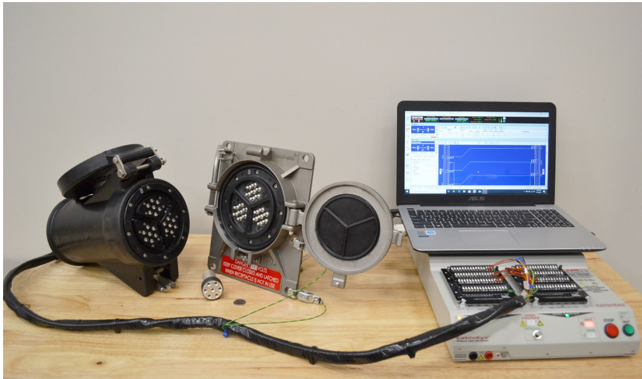
Figure 9 Cable tester set up with the shipboard plug and receptacle.
