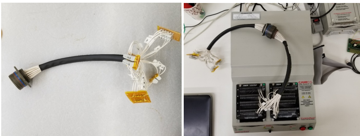
Figure 4 Surrogate shipboard shore power receptacle alone (Left) and connected to the surrogate plug, which is connected to the tester (Right)
