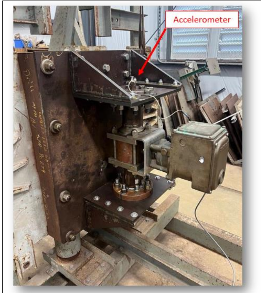
Figure 6: Test Arrangement Highlighting Accelerometer
