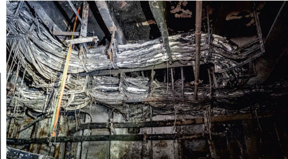
Damaged cableways published in Command Investigation into the Fire Aboard BHR
