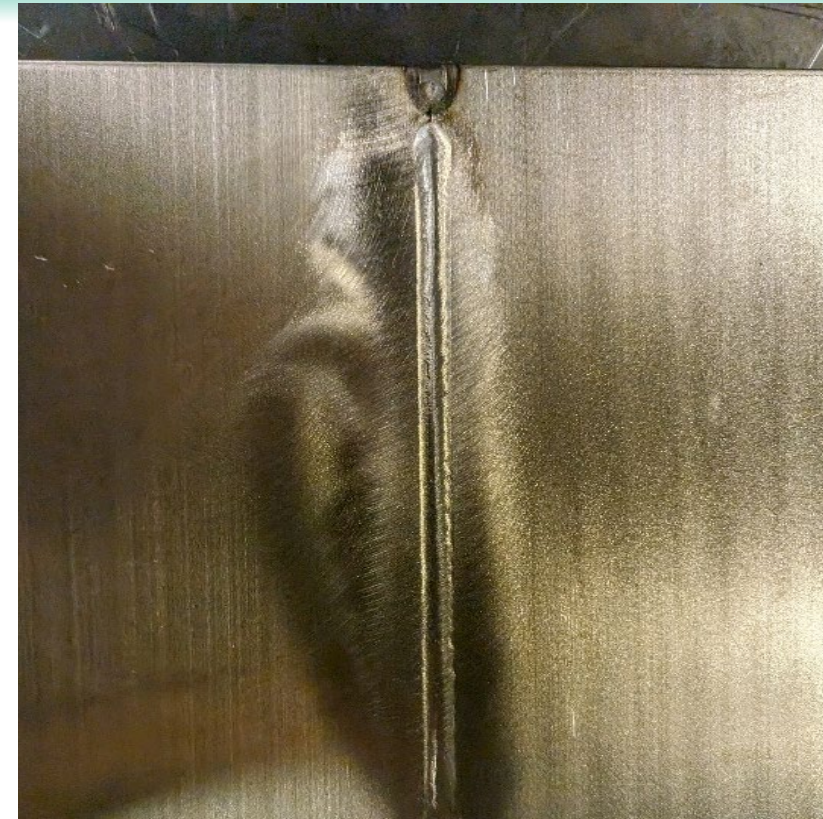
Satisfactory Seam Weld for Material D
