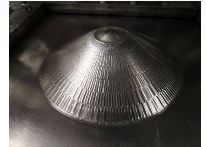
Multi-scale metamorphic manufacturing technology demonstrated for production of conical forms with drag-reduction riblet features for UUV applications
