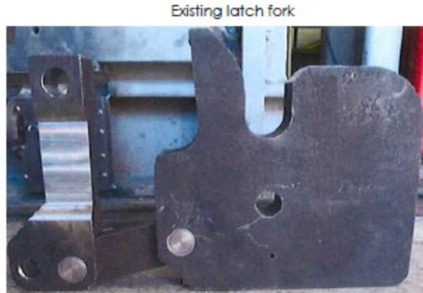
Latch fork with eccentric bushing and locking mechanism
