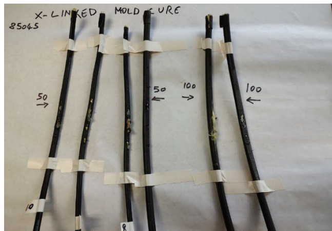
Thermoset Mold Cure X-Link (Fail @ 50 to 100 Cycles)
