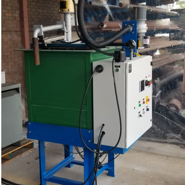
Above: Melting pot with transfer pump with stand attached Right: Prototype system at ARC Specialties facility in Houston, TX Below: Rendered drawing of prototype unit nested on skid
