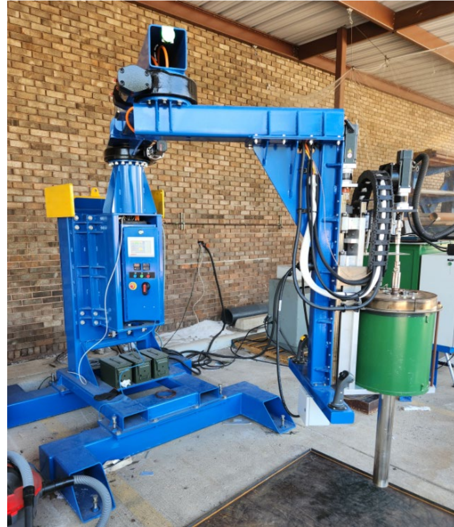
Above: Melting pot with transfer pump with stand attached Right: Prototype system at ARC Specialties facility in Houston, TX Below: Rendered drawing of prototype unit nested on skid
