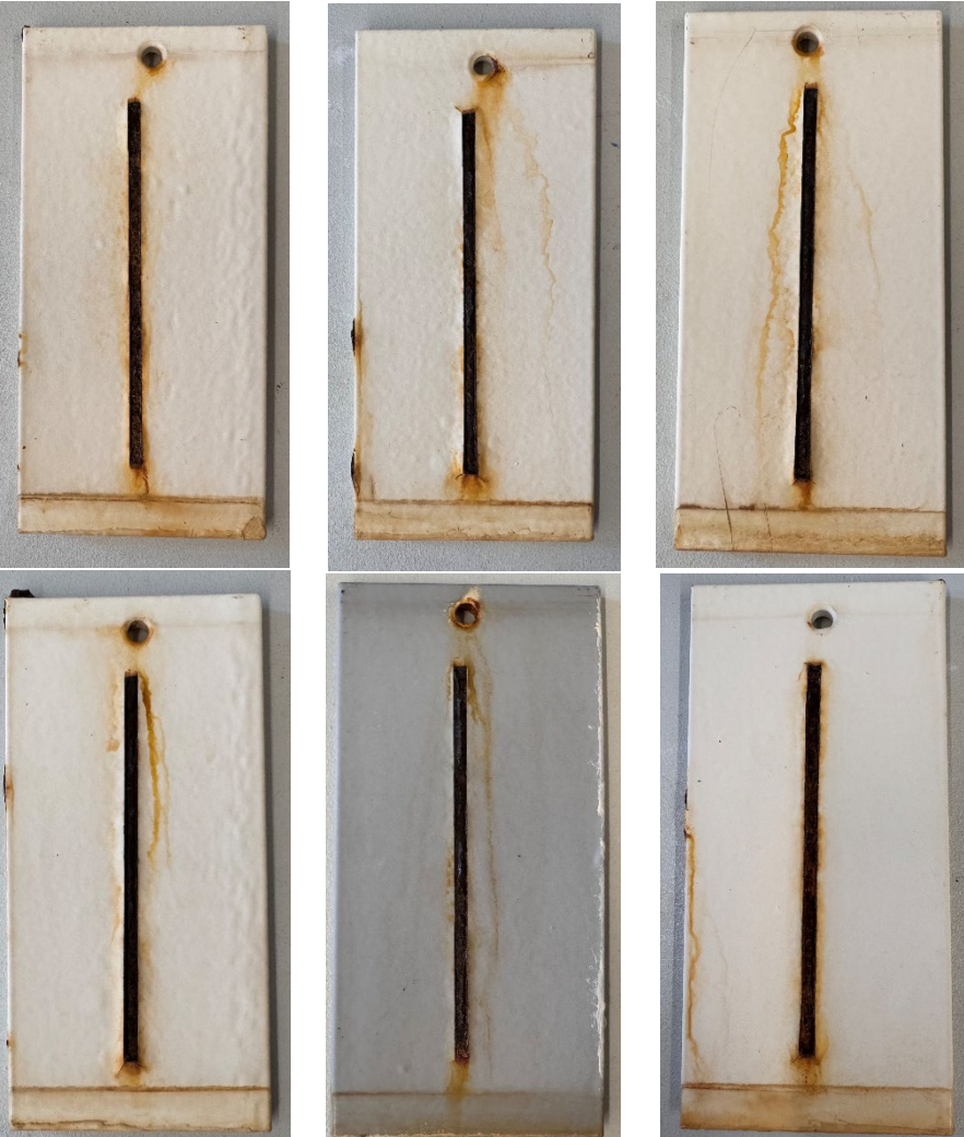
Accelerate Cyclic Corrosion
