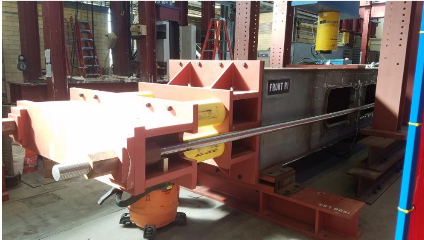
(left/right) Reinforced Opening Specimen #1 Installed in the Test Fixture and Tested
