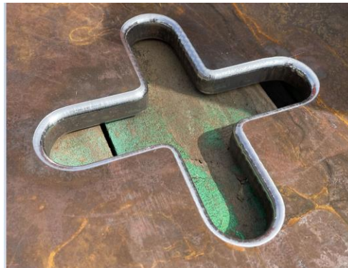
Ingalls cut vehicle lashing tie down in 1" plate
