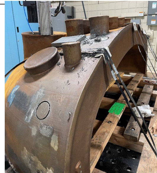
PM-HIP Scaled SMR Head and Valve body
