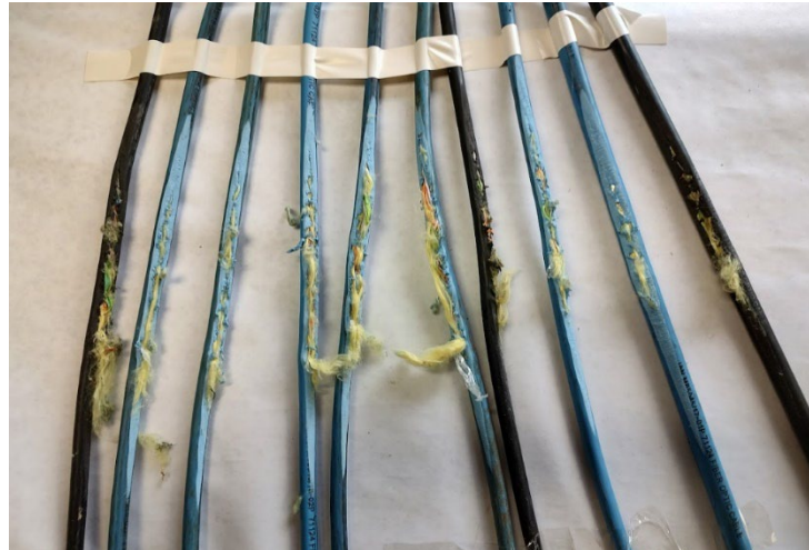
Thermoset Irrad X-Link (Fail @ 50 Cycles)
