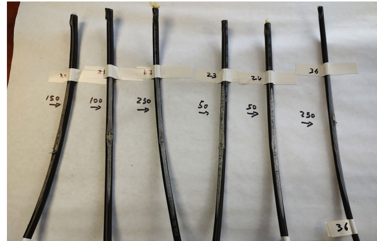
Thermoplastic (Fail @ 50 to 250 Cycles)
