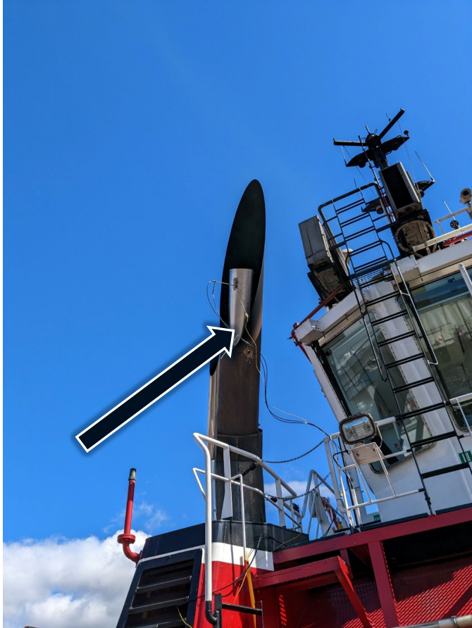
Exhaust modifications for accurate emission rate measurements
