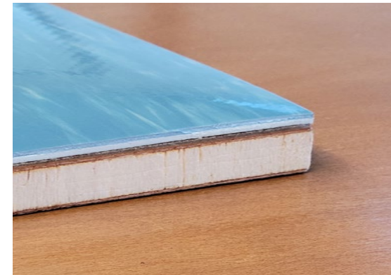
Phenolic Infused Balsa Wood Core with Lonmat Wear Surface
