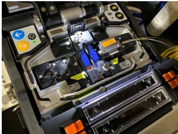
Figure 17. Fiber Loaded into Fusion Splicer
