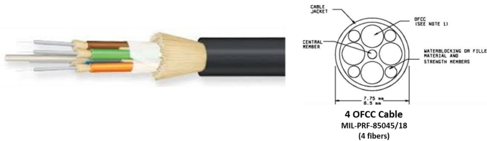
Figure 1. M85045 Cable Example (Single OFCC, 4-Fiber Cable)
