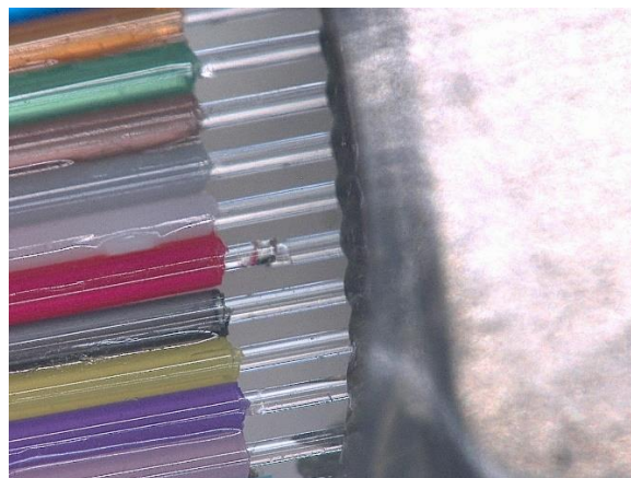
Figure 22. Cable A-1, Broken Fiber #7 (red fiber)
