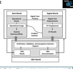
Verification: "Did we build the digital twin system right?" Validation: "Did we build the right digital twin system?"
