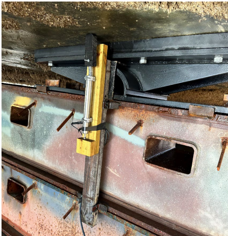
Figure 2: Linear Position Sensor Against Ship Hull
