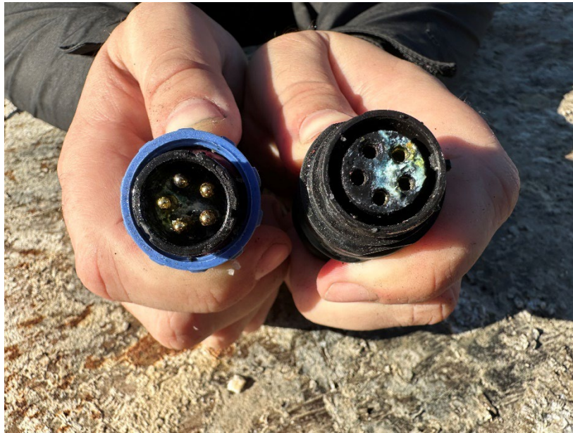
Figure 15: Connector condition post undocking. Showing possible water entry.
