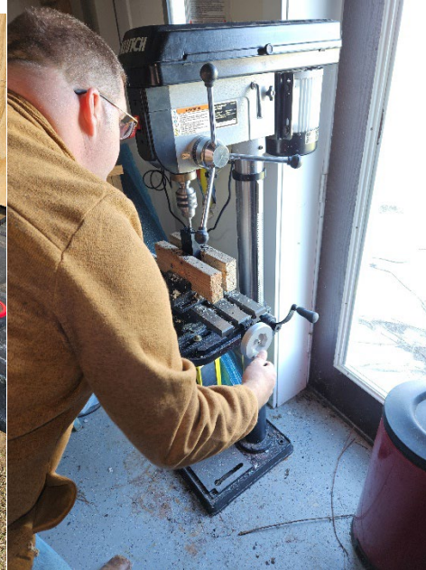
Figure 5: DMC machining HDPE probe
