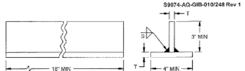
T = MAXIMUM THICKNESS TO BE USED IN PRODUCTION OR 3/8 INCH, WHICHEVER IS THE LESSER.
