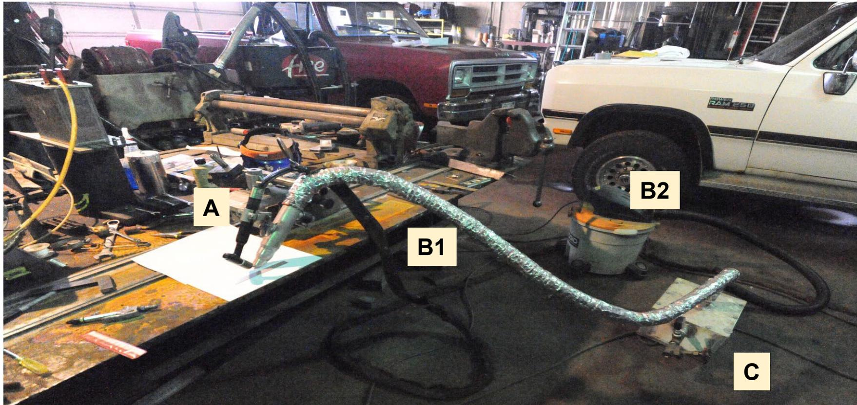
Key: A-Heat Source, B1-Vacuum Nozzle, B2-Vacuum, C-Capture Chamber
