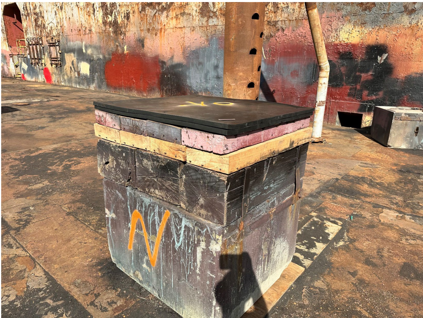
Figure 7: Docking 2 Neoprene Side Block
