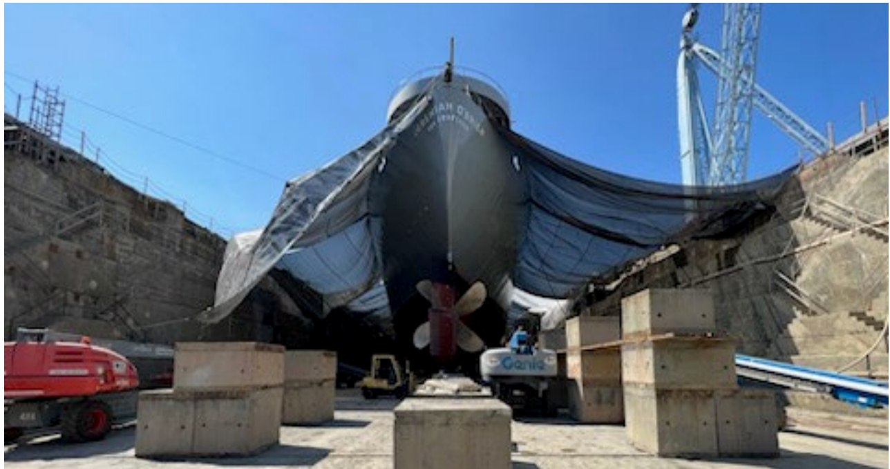
Figure 15: The block Fiber-reinforced block under USCG Cutter
