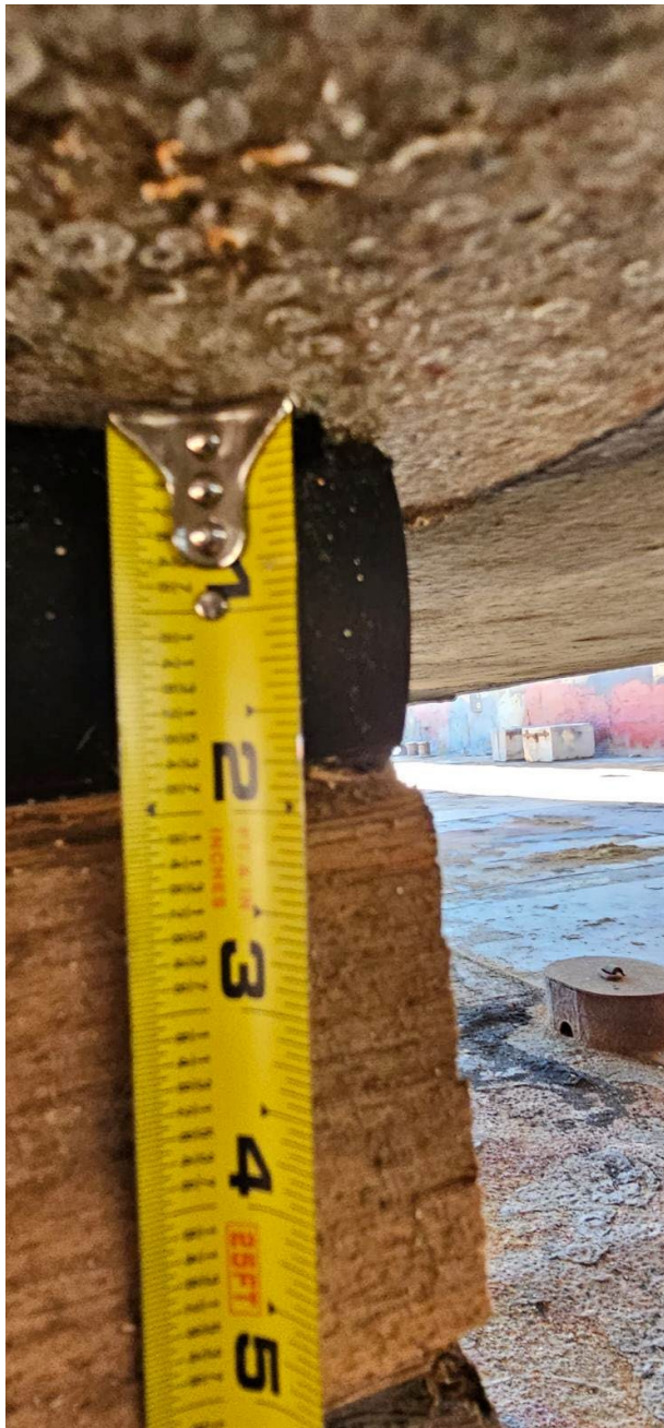
Figure 9: Docking 2 Neoprene Side Block Loaded Showing \frac{1}{4} " Compression
