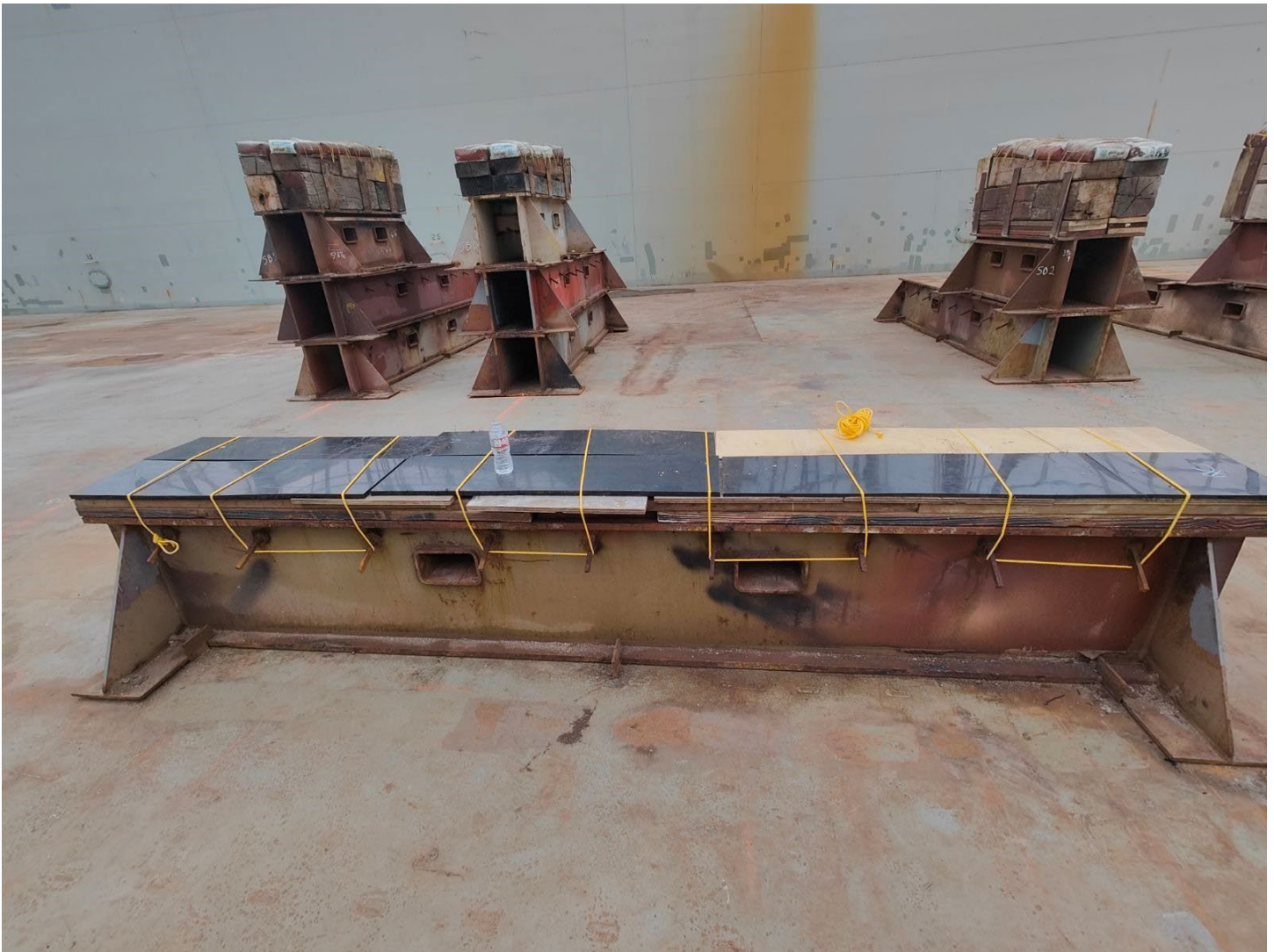
Figure 1: Docking 1 Keel Block
