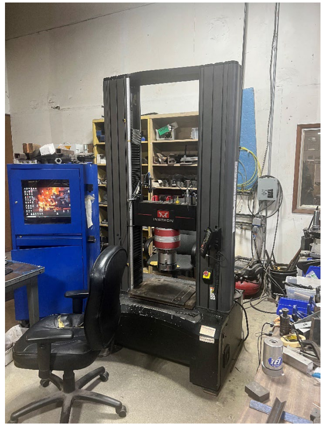
Figure 21: Equipment Used for Splitting Tensile Tests
