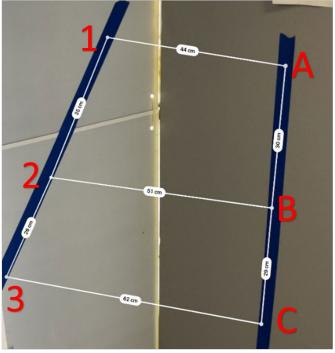
1cm accuracy constraint is ARKit default Lab results consistent with 1cm accuracy Optimal scan distance 10cm and 5m
