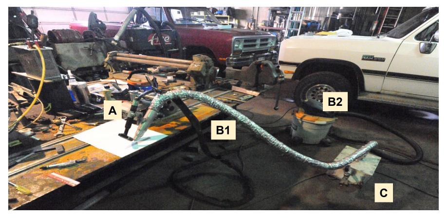
Key: A-Heat Source, B1-Vacuum Nozzle, B2-Vacuum, C-Capture Chamber
