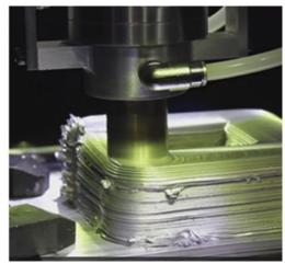
Scaling Up of 3D Printed Castings (NASSCO)
