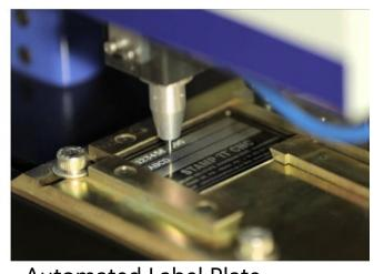
Automated Label Plate Generation (SSI) Benefit: Develop a process to reuse existing data already contained within the 3D design model for label plates.
