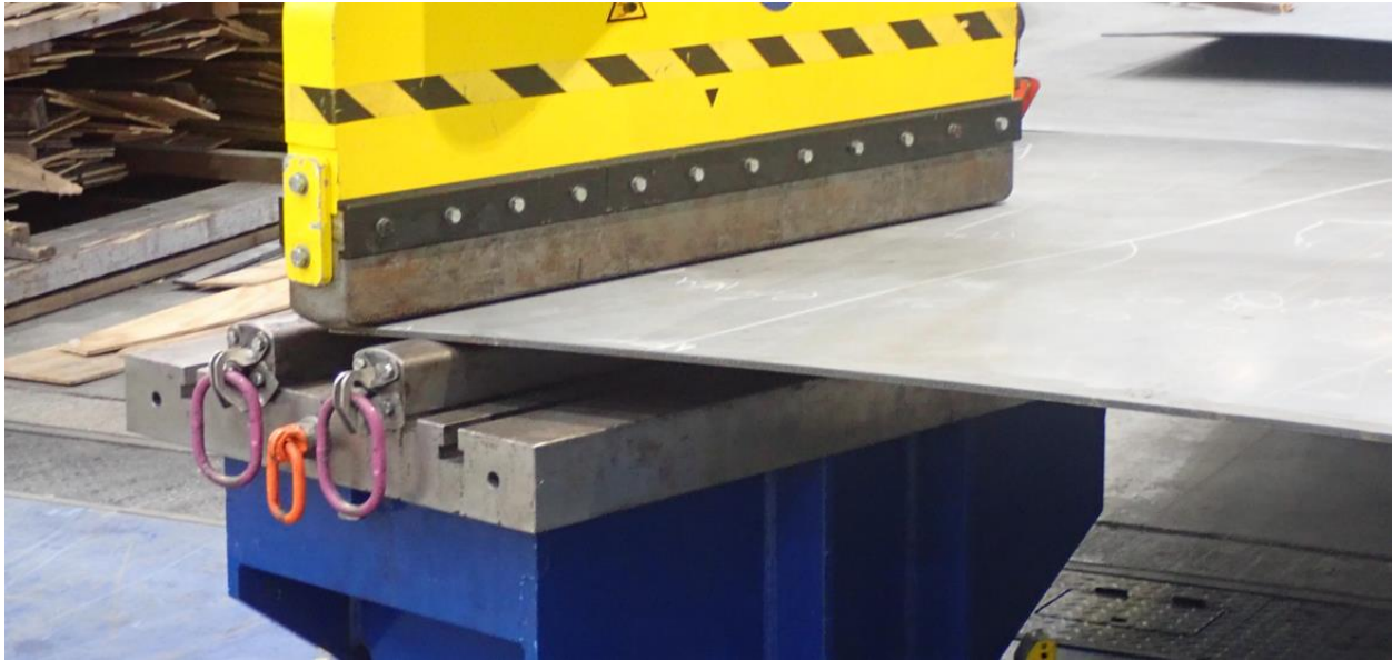
Figure 8: Forming Complex Curvature Using Punch Die
