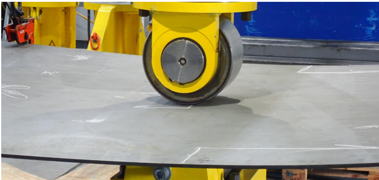
Figure 7: Plate Stretching Using English Wheel
