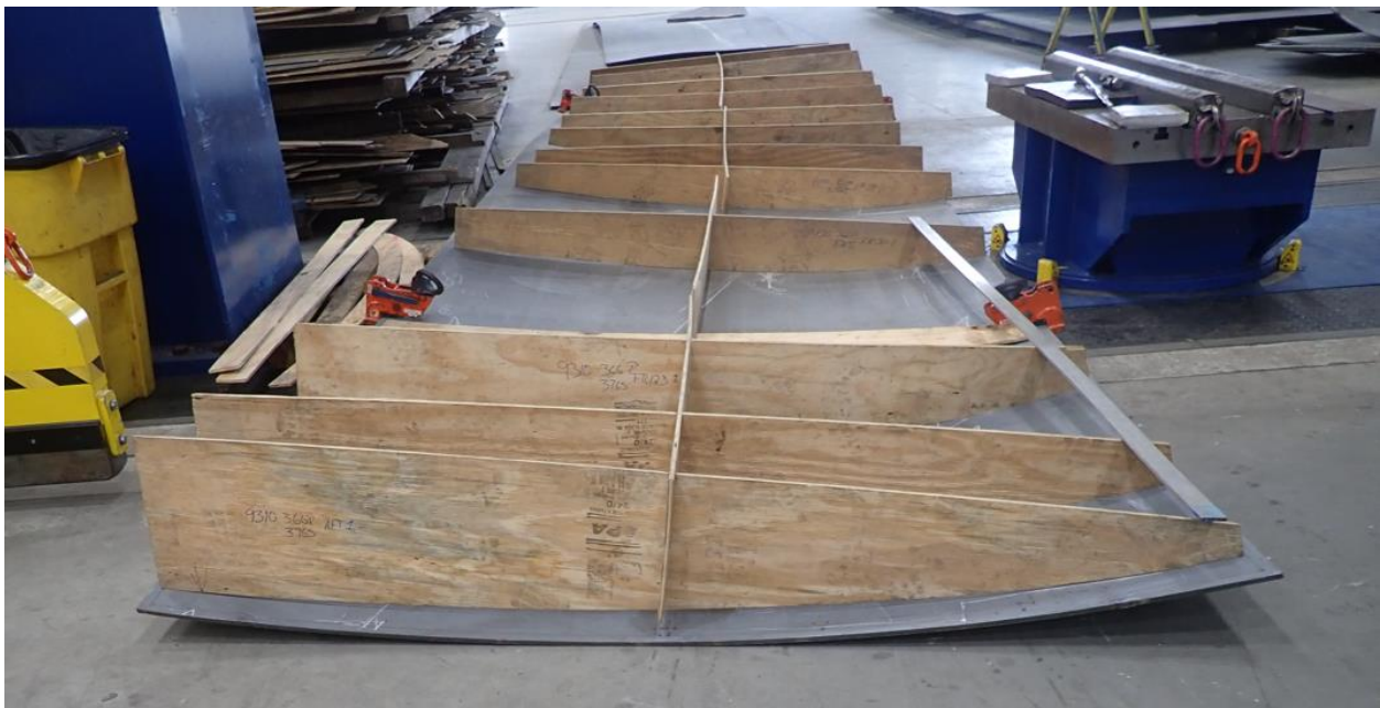
Figure 9: Final Shape of Plate with Edge Elongation
