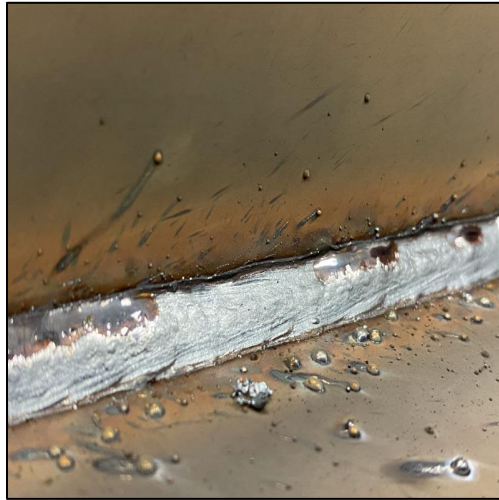
Figure 24. Excessive Spatter from the 100% CO 2 Test
