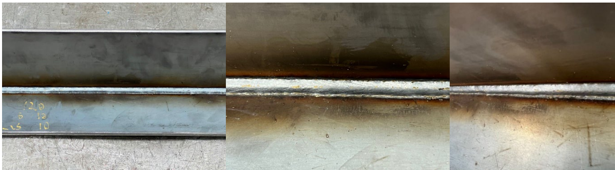
Figure 28. CLOOS Tandem Plate Welds
