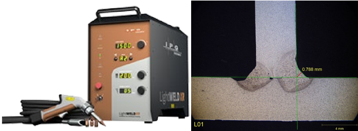
Figure 31. IPG LightWELD System, left, and Macrograph, right
