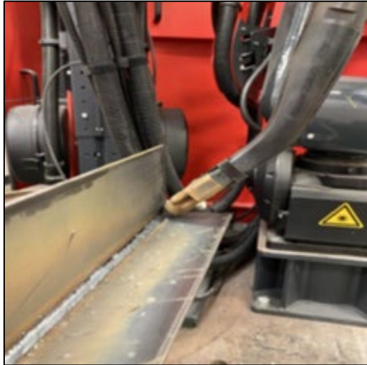
Figure 23. Fronius TPS/i TWIN Torch and Plate Setup
