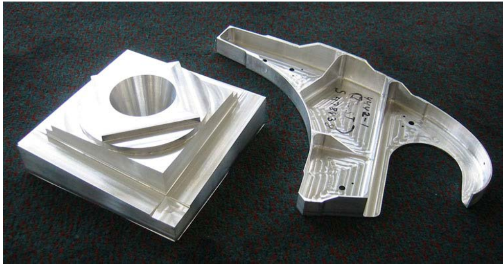
Figure 4-4 STEP-NC CC1 5-Axis test Parts
