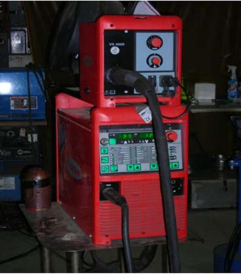
Fronius Transpulse Synergic 3200 power supply and Feeder
