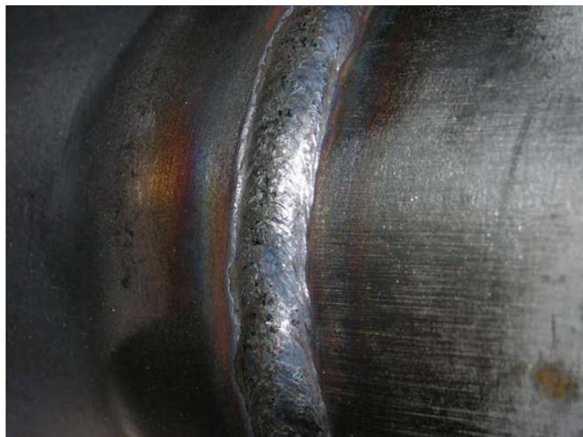
FIG. 5, Completed Production Weld on CRES Pipe
