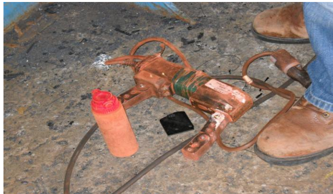
Figure 5a - MPI test equipment showing yoke and indicator spray
