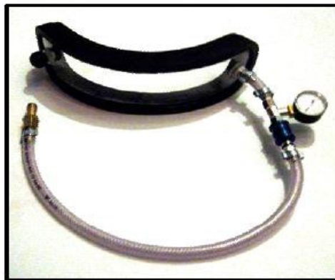
Figure 6 – Curved vacuum box used for pipe penetration assemblies (example shows large diameter)
