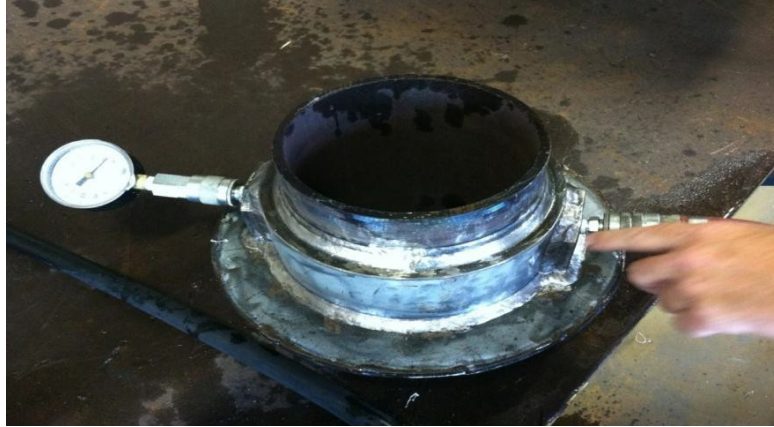
Figure 18b – First iteration of NASSCO fillet weld air test fixture (image)
