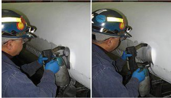
Figure 3a - A NDT technician performs MPI on a pipe to check for stress corrosion cracking
