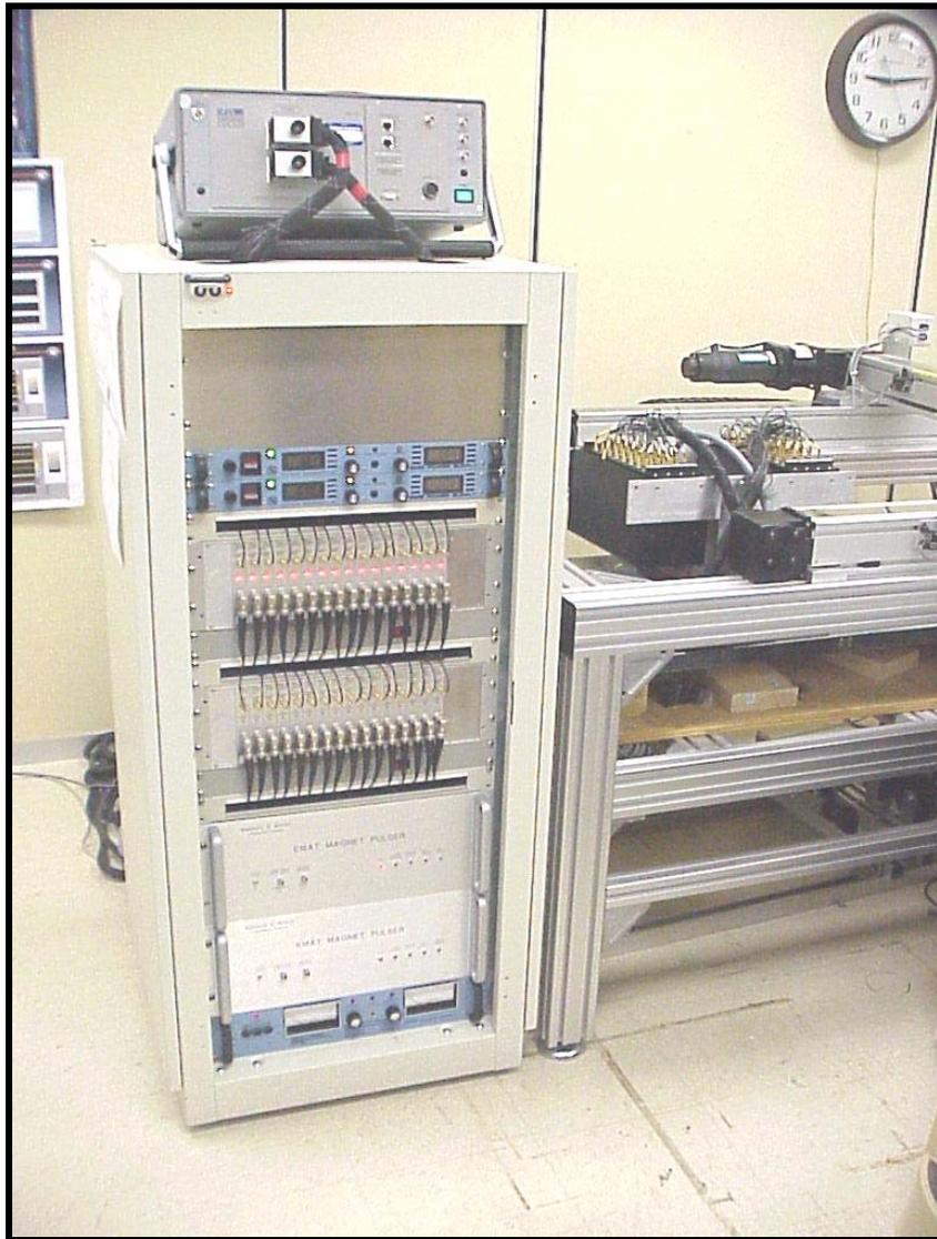
**Figure 9 - Phased Array EMAT System**
