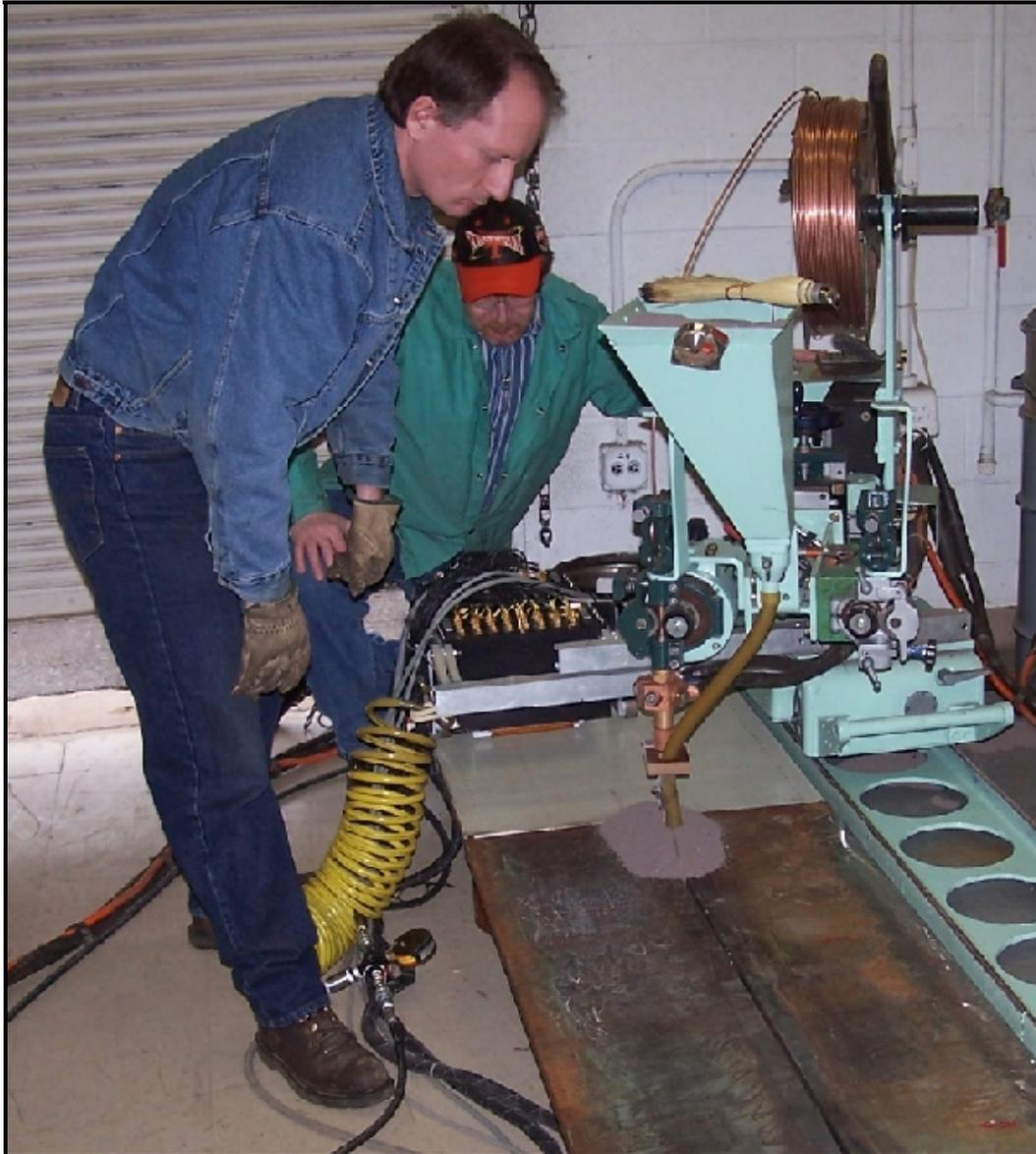
**Figure 23 - Portable Welder with EMAT Test Head Attached**
