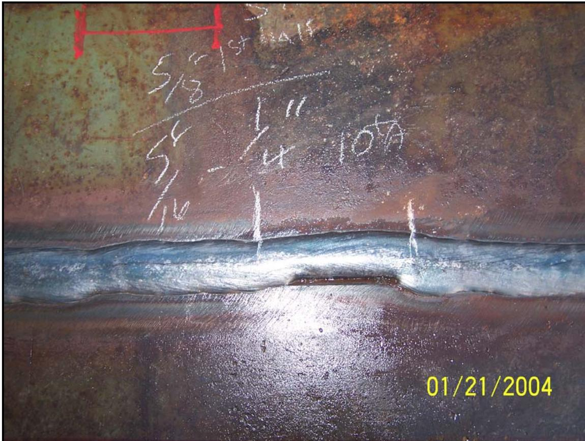
Figure 30 - Sample 1 Side 2 Photo Showing a Region Where the Torch was Moved off of the Joint.
