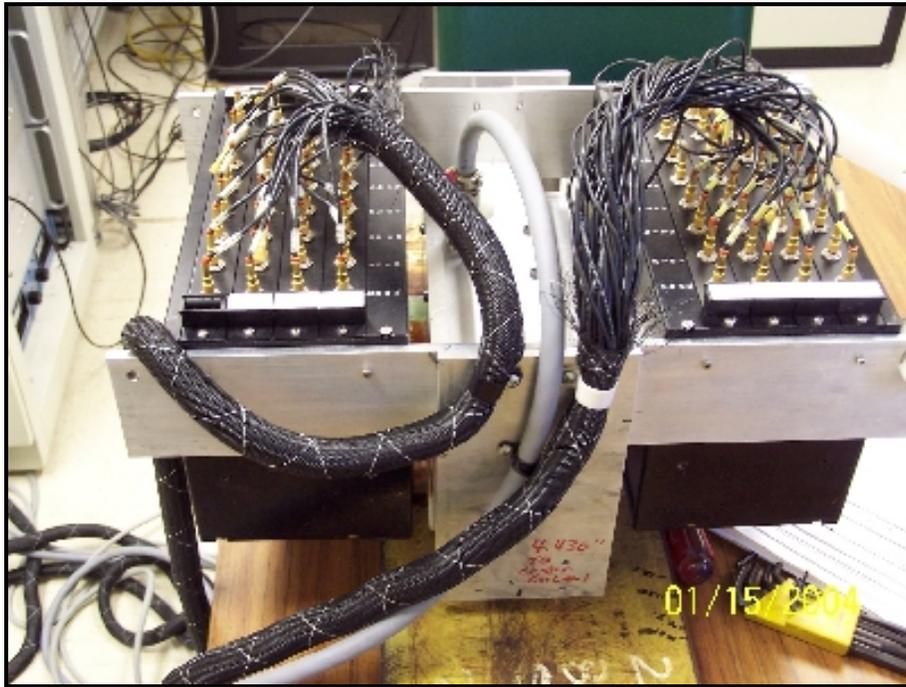
Figure 11 - EMAT Probe Head (Top View)
