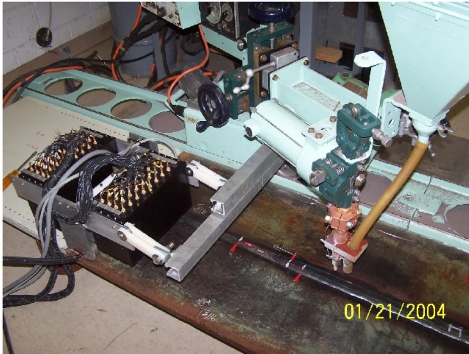
**Figure 24 - EMAT Head Attachment to Portable Welder Tractor**
