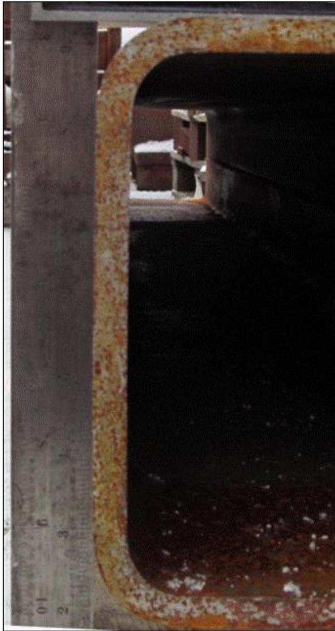
**Figure 9. Symmetry in the HFRW Tube Deformation after Fatigue Testing**
