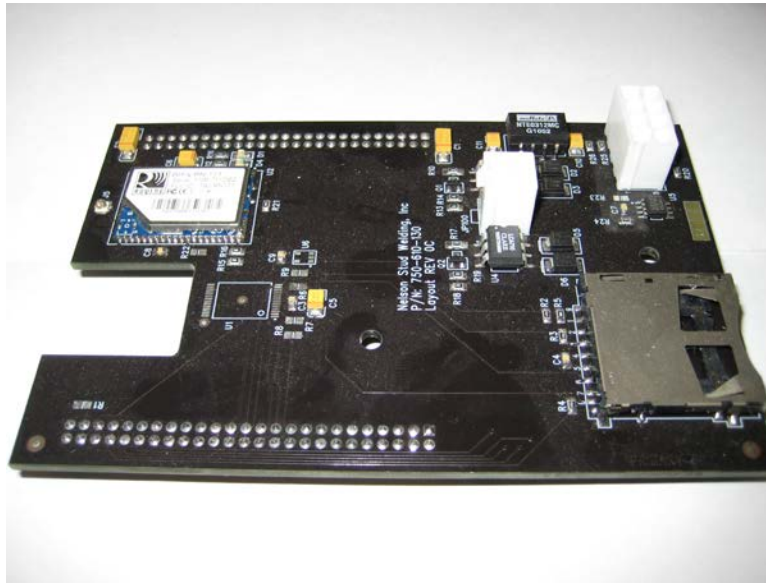
Figure 1. Daughter board for weld data storage in Nelson inverters
