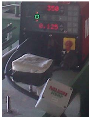
Figure 2. Weld counter mounted on weld cable
