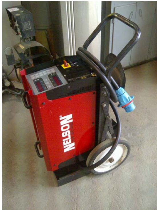
Figure 14. Motorized gun N1500i system on a mobile cart at Ingalls
