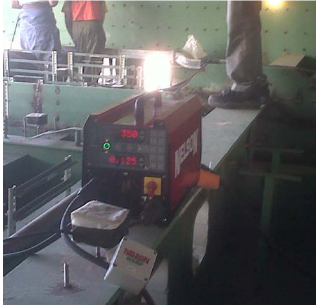
Figure 10. N800i with weld counter box at Ingalls
