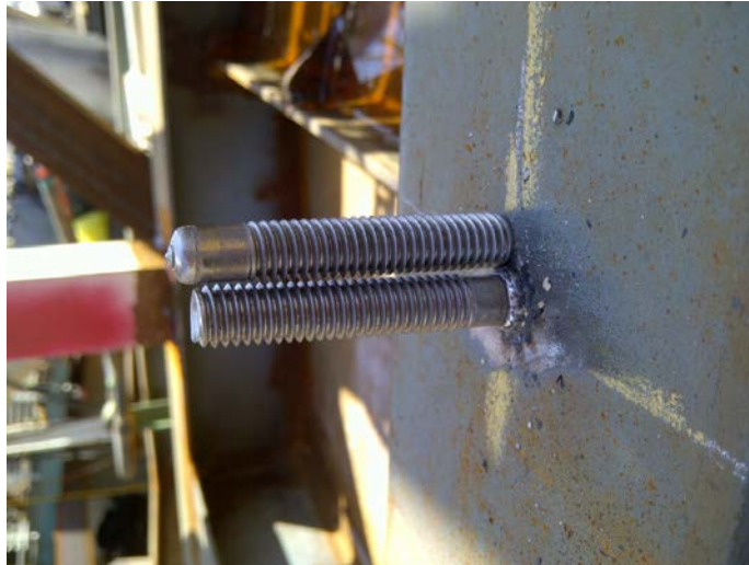
Figure 12. Burn-off measurement on a stud welded by a motorized gun
