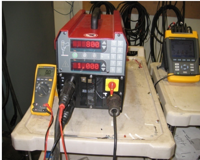
Figure 19. Nelweld 6000 with the Fluke power analyzer
