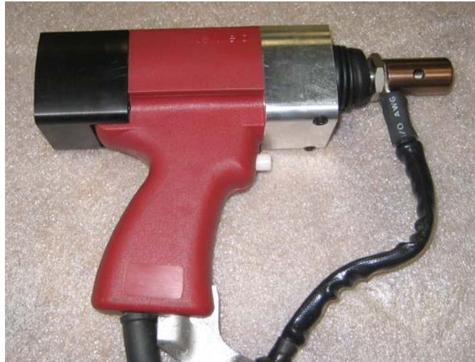
Figure 11. Motorized gun for 5/8" welding at Ingalls
