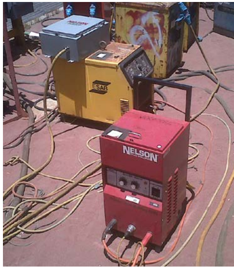
Figure 8. Series 4000 with energy meter box at Ingalls
