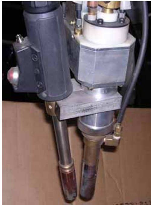
Figure 15. RLT-GMAW Torch Configuration (RE-GMAW torch is on the right.)
