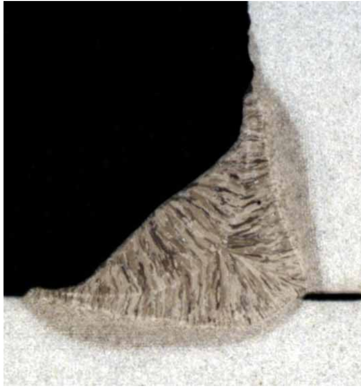
Figure 23. Cross Section of a 3-mm Fillet Weld Developed with 1.1/1.1-mm Diameter Electrode Combination using RLT-GMAW
