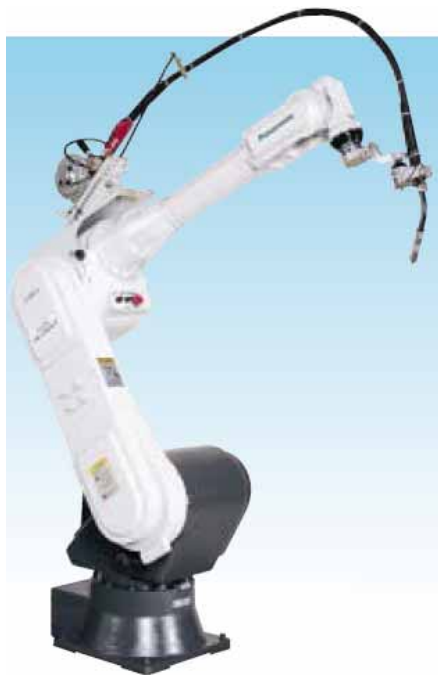
Figure 13. Panasonic VR-006 6-Axis Robot
