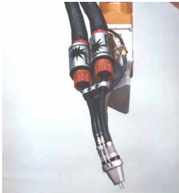
Figure 6. T-GMAW Torch (Note the close proximity of the electrodes.)
