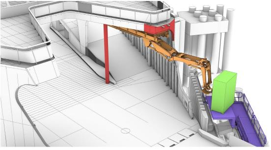
Arm extending during charging operations (cabling and covering not shown)
