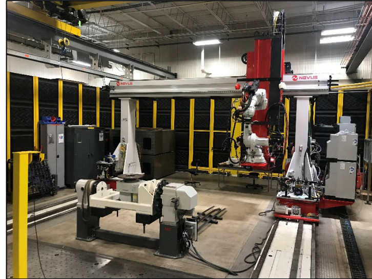
Large Scale Multi-Process Robotic Gantry DED System
