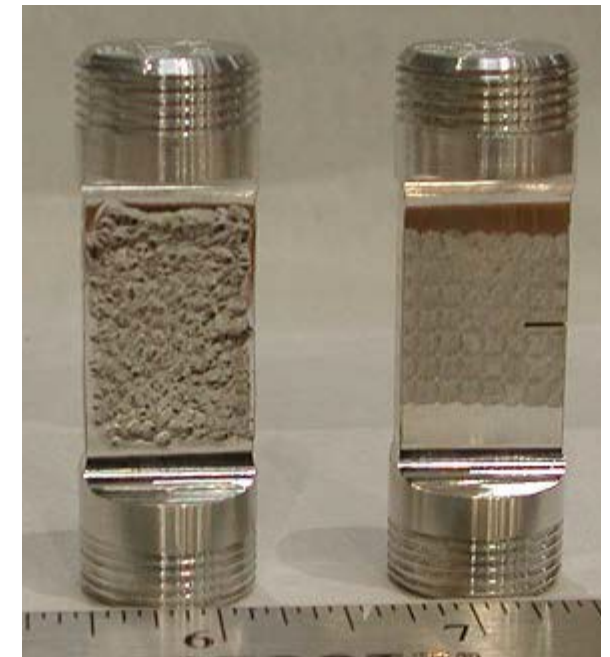
UIT surface (Left) vs LSP surface (right) at 1 GW/cm 2 (1-20-1):
