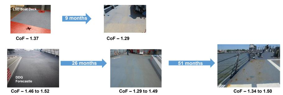
CoF of spray applied polysiloxane nonskid on in-service steel decks maintaining CoF and service life limited by mechanical damage.
