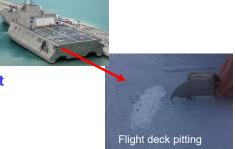
REQUIREMENTS: FY-22, Change 1, Standard Item 009-32, Table 2, Lines 55 & 56 require application of either MIL-PRF-24667C, Type I or Type V nonskid on flight deck surface preparation in accordance with:
