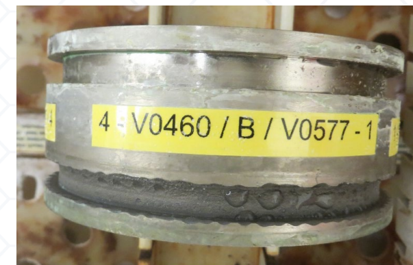
Upper ring – repaired Lower ring – not repaired 100 hrs ASTM B117 Salt Fog
