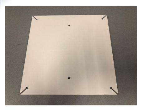
The Ultem Glass Fiber reinforced composite sheet is water jet cut from a large 4' x 12' sheet.
